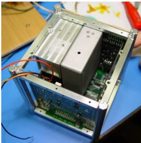
Figure 1.4: Picture of DTUosat during assembly. Bottom PCB: on-board computer (OBC) which serves as a motherboard. Lower side PCB: Radio. Left side PCB: Power. Upper side PCB: Payload. Right side PCB: Attitude Control & Determination System (ACDS). A sun sensor is included on each side panel except on the payload side. The two metal cases are housings for the two payloads: a camera (left) and an electrodynamic tether (right).
